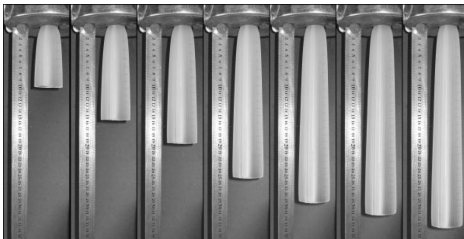
Figure 2 Typical parison images taken at a sequent time.
